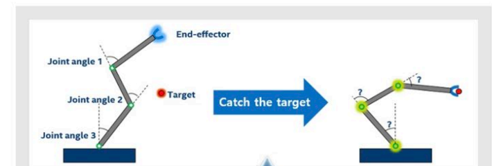
Figure 1. An example of inverse kinematics. The left robot arm has three joint angles, one end effector, and the target object. The right robot arm must determine the joint angles to move the end effector to the target object.
